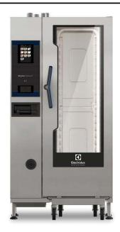
219703 (ECOG201T3O30) SkyLine PremiumS Combi Boiler Oven with touch screen control, 20x1/1GN, gas, 3 cooking modes (automatic, recipe program, manual), automatic cleaning, spray gun, 6-sensor probe, 3-glass door and IoT module -120V US
